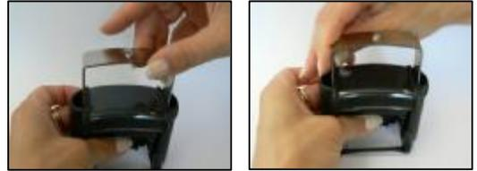
14. Once attached move the metal frame up and down several times to insure that it moves freely and that the die plate is in the correct position.
