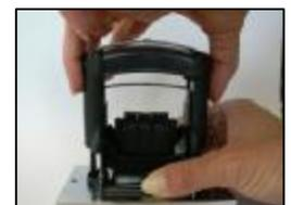
6. Remove axle and lift out band assembly with cam frame from internal metal frame.
