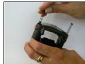
17. Make sure that the springs go into the spring channels on each side and that the metal frame is completely matched up with the plastic handle.
