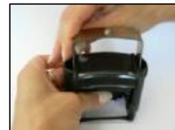
5. Remove plastic frame cover from internal metal frame; you may need to release the bottom of the plastic frame from the internal metal frame by applying slight outward pressure.
