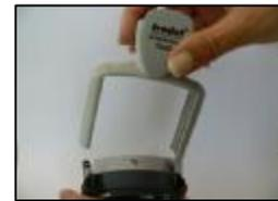
4. Remove inside metal frame; it will be necessary to apply slight outward pressure to release the axle.
