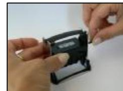
12. Replace plastic cover frame (still lifting up the assembly) and push down until it locks into base of internal metal frame.
