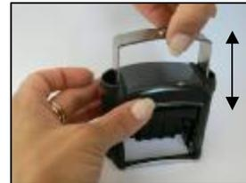
15. Make sure that the locking buttons are in the out or unlock position. You may have to use a screw driver to move them to this position.
